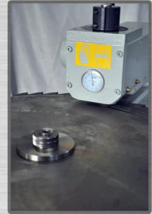
Hydraulic Tensioning Control by Hydraulic Gauge
