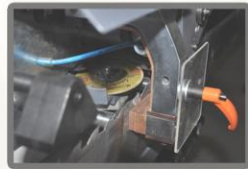
Automatic Stellite rod cutting by angled grinder.
